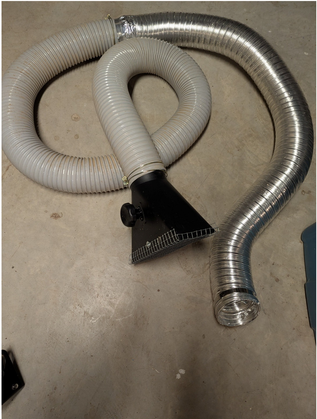
Dust collector hose and hood
